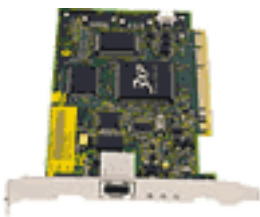
An image of a Fast Ethernet network interface card.
